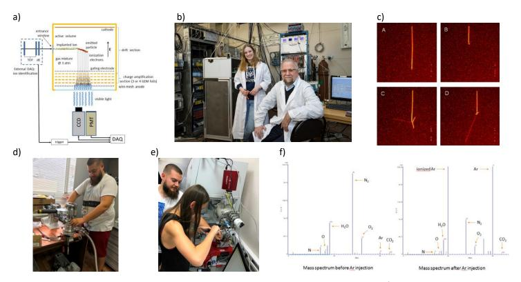
a) The scheme of the OTPC operation b) The OTPC installed at the ACCULINNA beam line c) example picture of decay of <sup>9</sup>C [A. Giska, Bachelor thesis, UW, 2018] d) students at work – construction of a vacuum stand e) preparation of RGA system for gas mixture contents analysis f) example spectra of the gas mixture contents measured with RGA.
