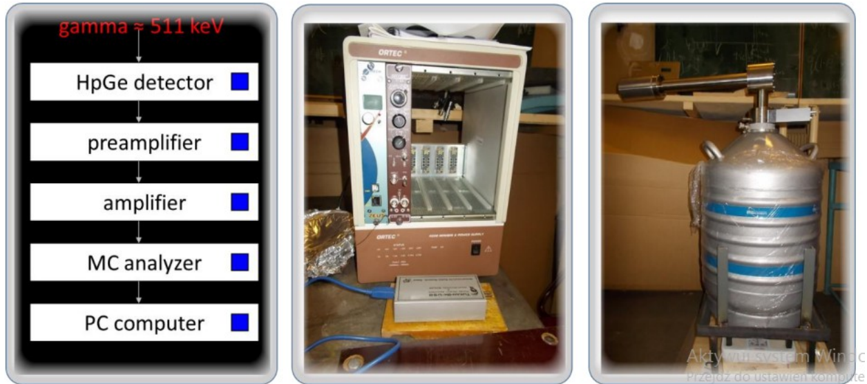
Fig. 2 Positron Doppler broadening spectroscopy equipment.
